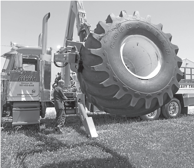
Seth Hartle of Mike’s Repair of Owatonna, demonstrates how their new tire repair truck, designed for heavy equipment, can squeeze a tire up to 102 inches wide.
