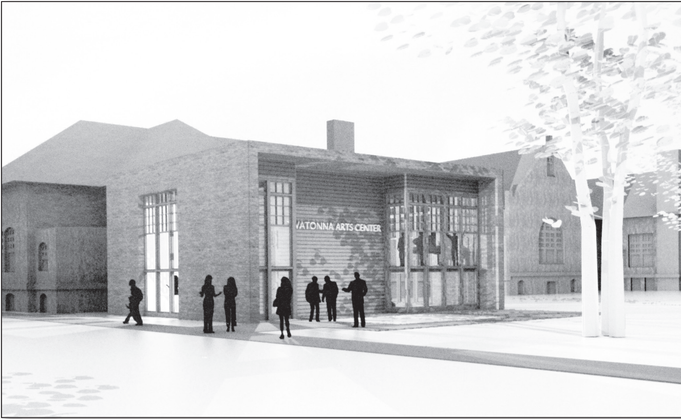
Staff photo by Shannon Kinley This is what the new Owatonna Arts Center entrance should look like after it is completed. The entrance, designed by BKV (Boarman Kroos Vogel) Group out of Minneapolis, will feature a front desk and welcoming area, an expanded entrance, an additional display area, a door to the lower level and an elevator.
