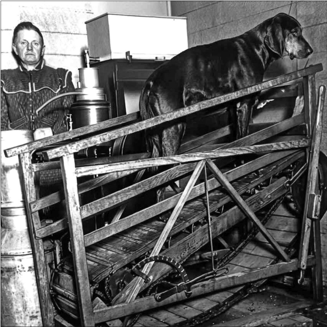
Mina Holmes is shown operating her “dog-powered” cream separator she developed in the early 1900s. The unit is now on display at the Steele County Village of Yesteryear in Owatonna.
